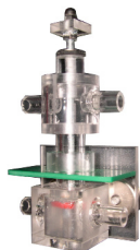
Hydrant at pipeline network
